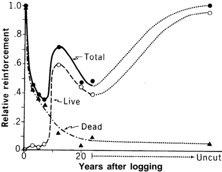
**FIGURE 3.** *The relative reinforcement of soils by live roots generally increased while that by dead roots rapidly decreased with increasing time after clear-felling. The total reinforcement by live and dead roots dropped to a low point about 7 years after logging.*
