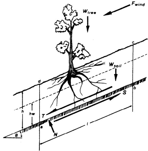
Figure 6. Part of a forested infinite slope showing forces operating on a sliding soil mass.
