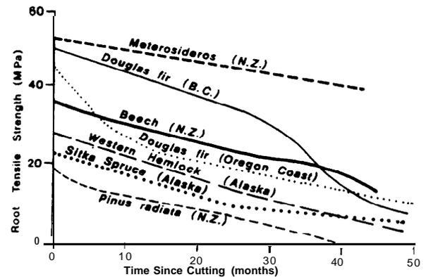
Figure 4. Curves of mean tensile strength vs time elapsed since tree felling for small roots of various conifer and hardwood trees,
